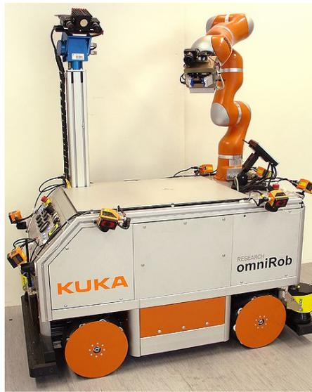
Figure 3.1: The KUKA omniRob without (left) and with (right) the modifications of the DLR. Source: DLR internal
